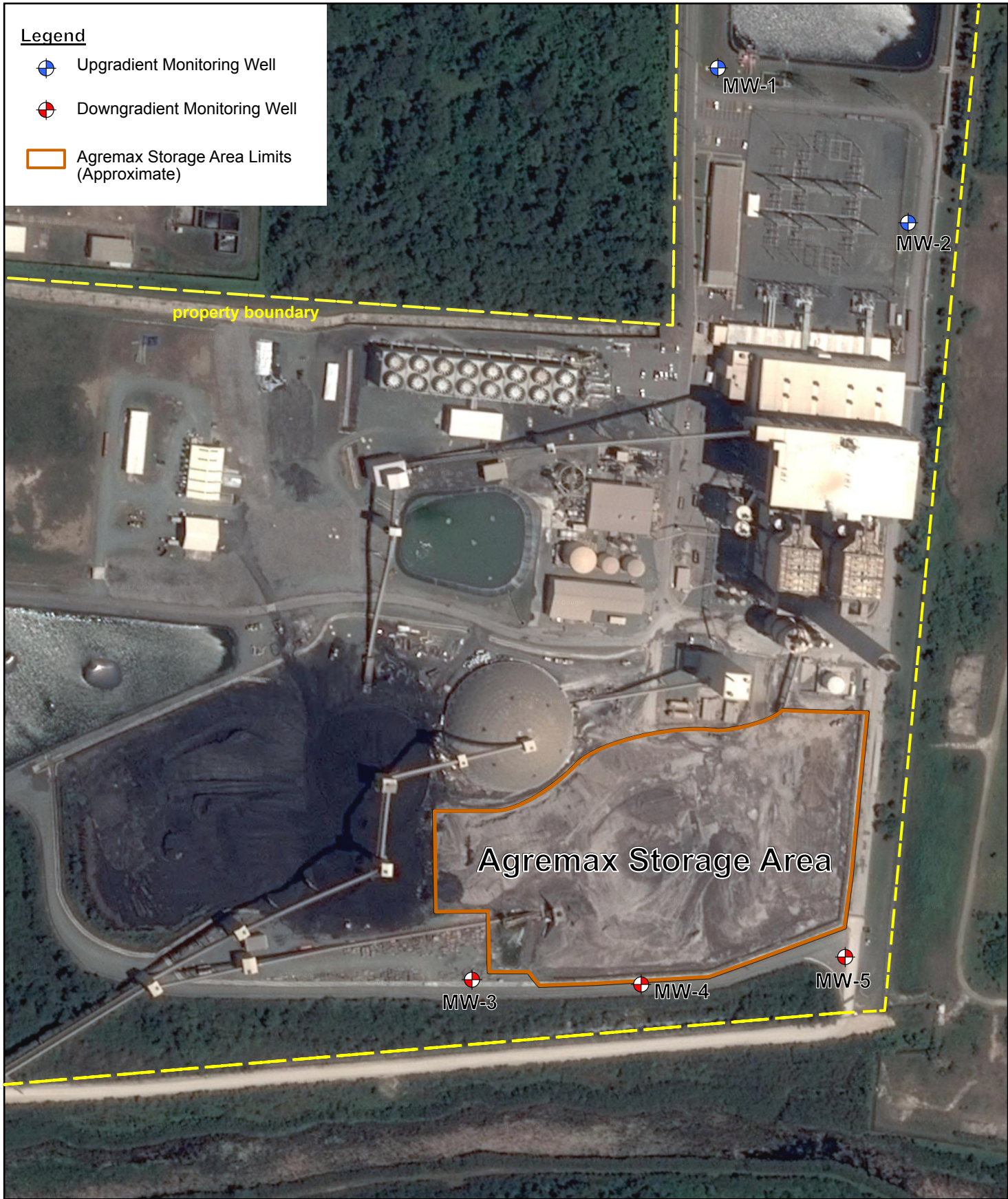
Figure 2 Groundwater Monitoring System AES Puerto Rico, LP Guayama, Puerto Rico
